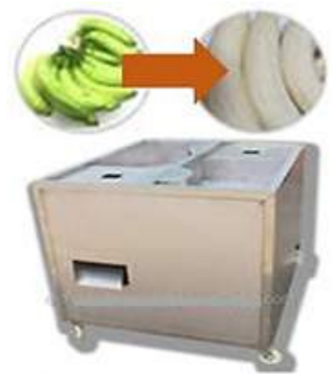
An industrial green banana peeler able to processes 600 units per hour
