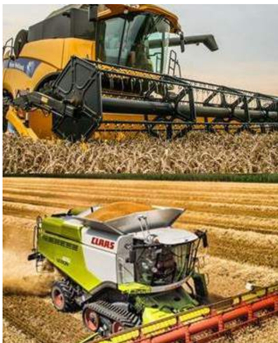
New Holland CX 8080 with 3.7 m cutting width (above) and CLAAS Lexion Combine 670 with a 12 m cutting width (below)
