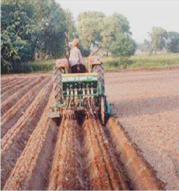
Establishing raised beds, furrows and planting rows in a single pass over a tilled and level field
