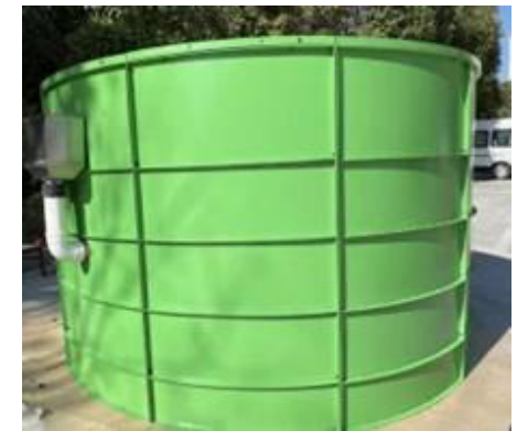
A batch digester for producing biogas from poultry manure
