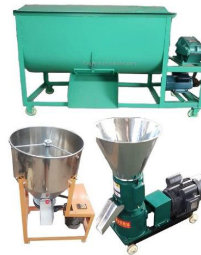
A horizontal mixer (top), mill (left) and pellet machine (right) used in small-scale feed production
