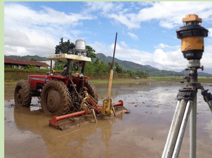
Laser-guided land leveling system with tractor.
