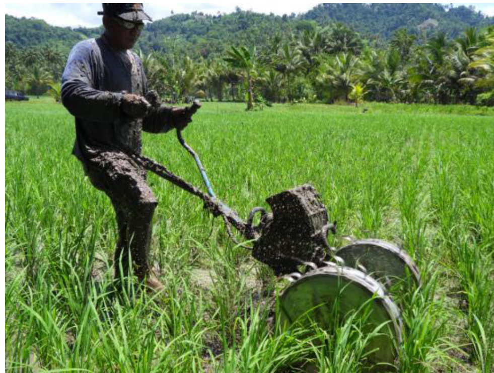
Rotary power weeder from AfricaRice.
