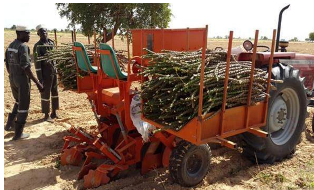
The Model 2AMSU two-row cassava planter being prepared for operations in Nigeria.
