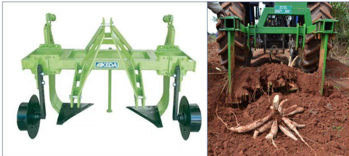
Harvesting attachments useful for cassava root lifting: An attachment from China (left) and a lifter in operation in Nigeria.
