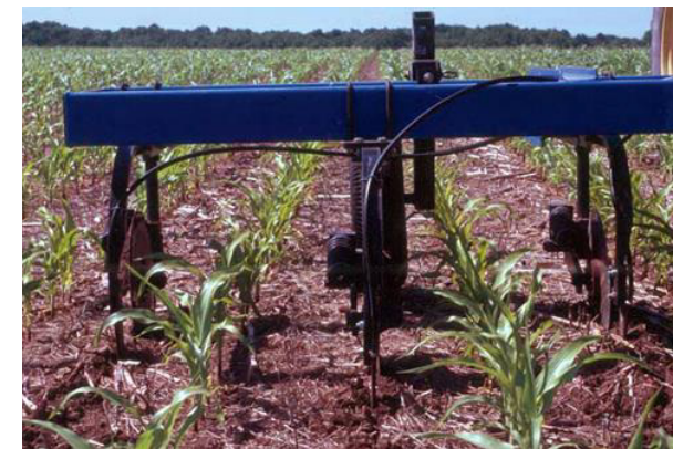
Tractor-mounted driller for N topdressing.
