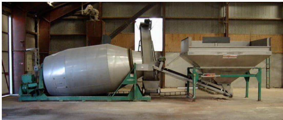
Dry rotary system used in fertilizer blending.
