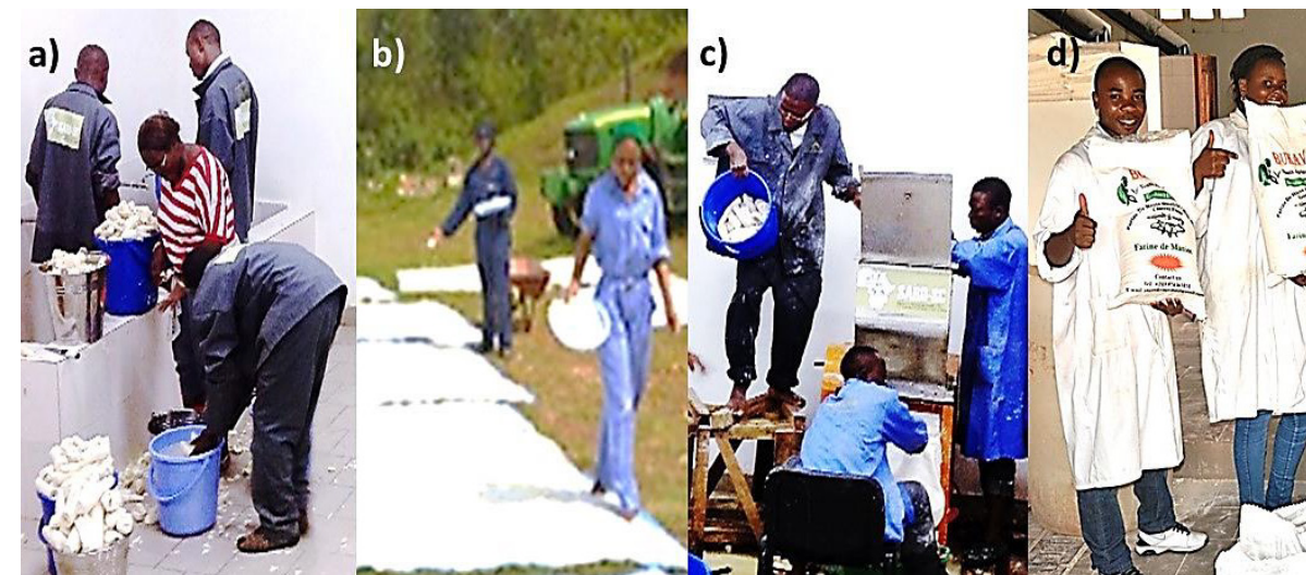
A "low-tech" youth-led cassava flour factory in action: a) washing and shredding peeled cassava roots, b) air drying shredded roots, c) milling dried roots into flour, d) displaying the finished product
