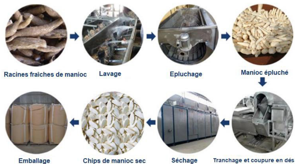
Steps of large-scale cassava chip production process
