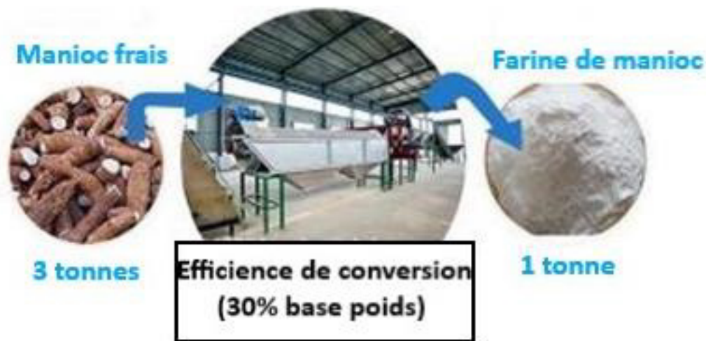
The conversion of fresh cassava root to high quality cassava flour
