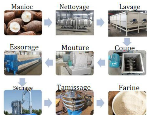
A modern industrial cassava flour processing approach where all operations are mechanized (from: cassavaprocessing.com )
