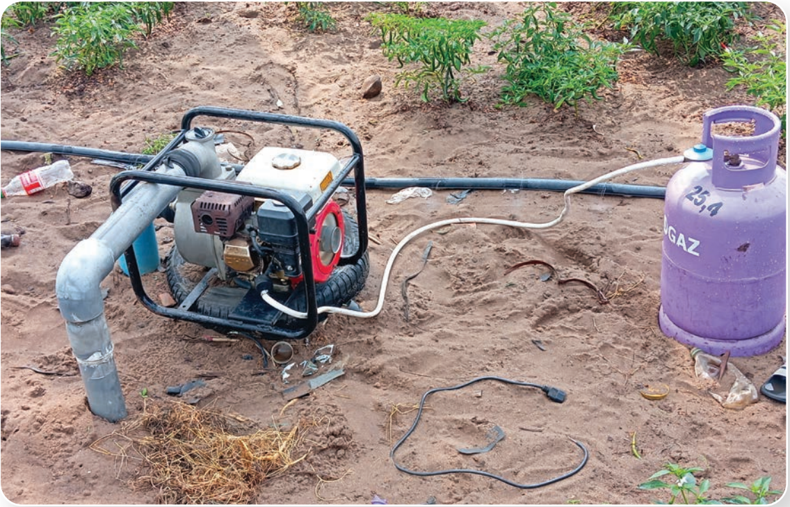
Figure 12: Power source for irrigation: a motor pump using domestic gas
