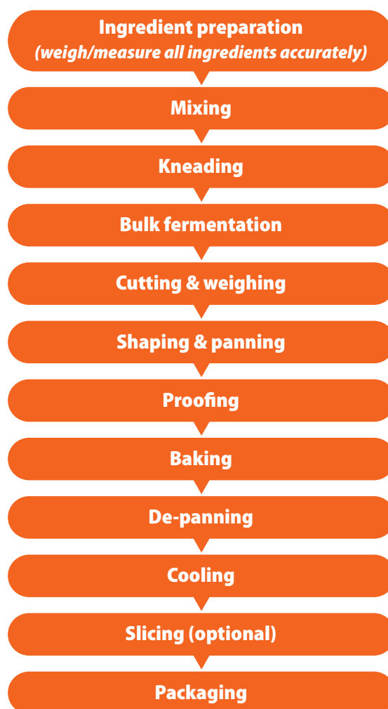
Figure 3.31. Sequence of bread production steps.
