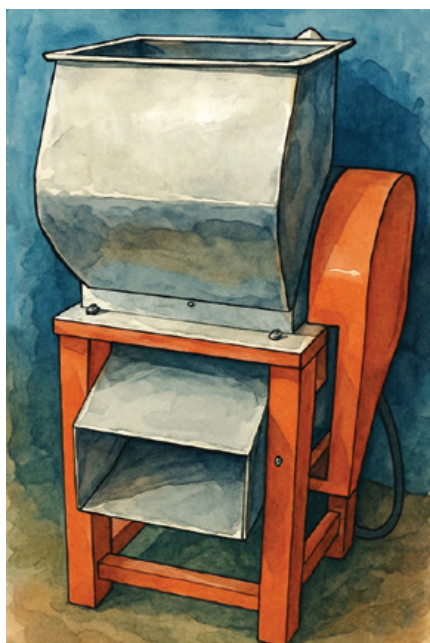
Figure 3.25. Mechanical cassava grater.
