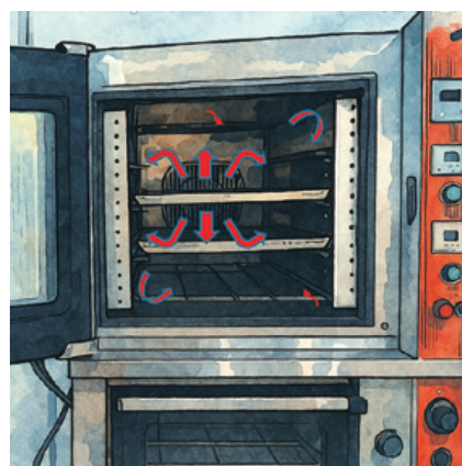
Figure 3.17. Air circulation in a convection oven.
