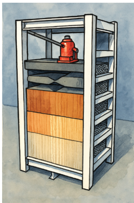
Figure 3.26. Cassava dewatering presses.
